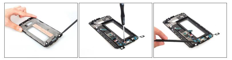
• Remove USB board. If you replace USB board only, please be careful with the LCD screen very much. Once a defect, the screen will be cracked or broken.
