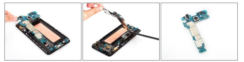
• Release USB board connector on the back and remove the motherboard.
