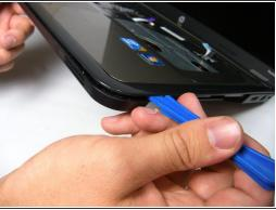
Use the plastic opening tool to pry out the front panel around the entire computer.
