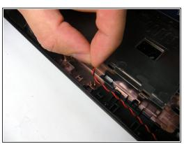
Locate the red and black speaker cables connecting the speakers and detach them from the two holders.
