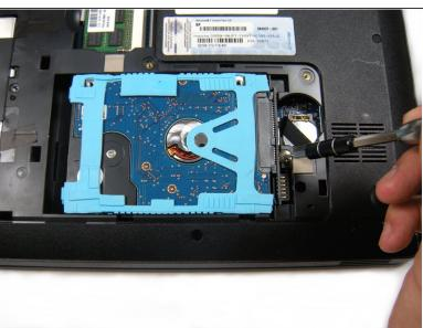
Use the PH 00 screwdriver to unscrew the 2.5 mm screw to the right of the hard drive.
