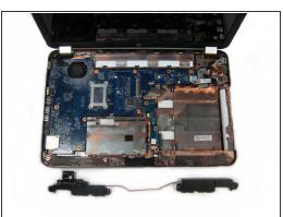
• Lift the right speaker directly up and remove it from the computer.
