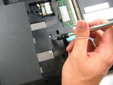
• Using the PH 00 screwdriver, remove the screw left of the CD drive.
