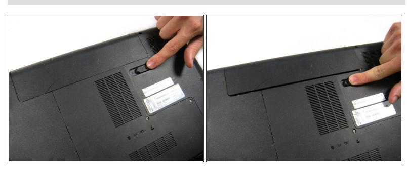
Slide the battery switch to the left until the battery unlatches from the base of the laptop.
