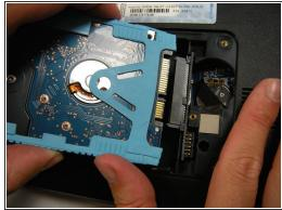
Pull the triangular blue tab to diconnect and remove the hard drive. You can see the word 'Pull' on the cover.
