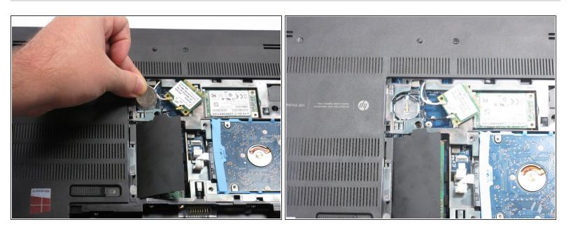
Remove the battery from the device.
