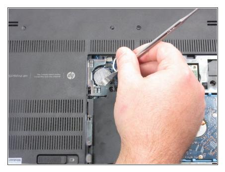
Use a plastic or metal spudger to release the CMOS battery from the clips.
