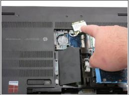
Remove the screw from the wireless adapter with a PH0 screwdriver then move the adapter out of the way to access the CMOS battery.
