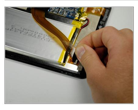
Remove the black tape covering the zero insertion force (ZIF) connector that holds down the end of the
