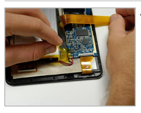
Carefully remove the yellow tape from the red and black wires connecting the battery to the motherboard.
