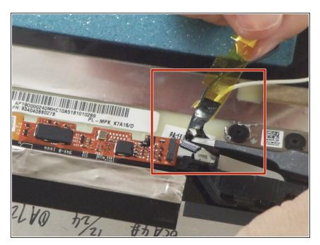
Use the tweezers to unplug the black connection near the hinge of the laptop, taking the yellow tape off with it.
