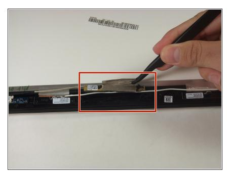
Use the tweezers to pull up the camera by simply pulling upwards on the tape that is over it.
