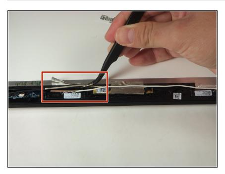
Use the tweezers to pull the tape upwards in order to free the wires underneath it.
