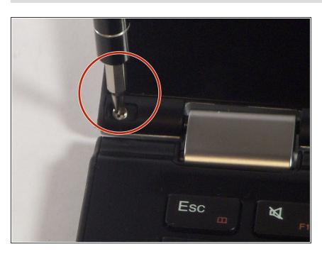
Remove the single silver 5 mm screw found beneath each rubber insert.
