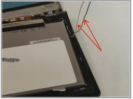
• Use the plastic opening tool to work the black component up and out of its original spot, then pull out the following connected wires.
