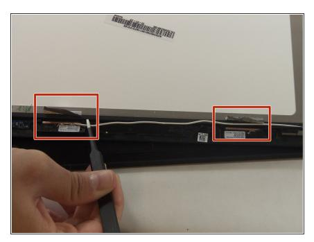
Use the tweezers to follow the wires and to pull them out from under the plastic black hooks. Also pull up any tape that is over the wires.
