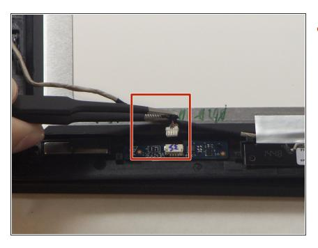
Use the tweezers to unplug the connector near the top of the screen.
