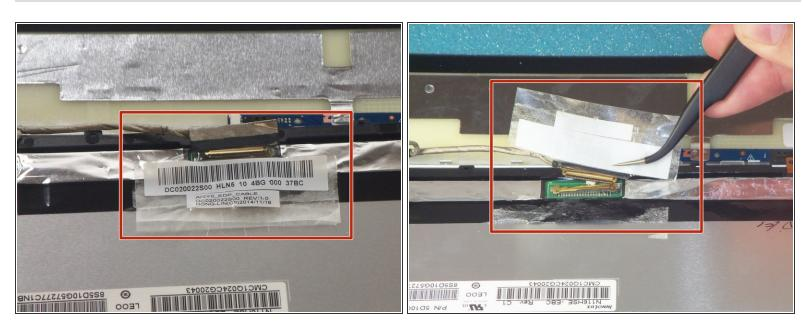
• Use the tweezers to pull the tape upwards. The tape will pull the wires up with it, separating the connection.
