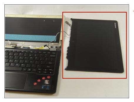
Gently lift and remove the screen for replacing.
