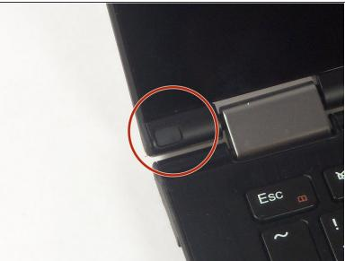
• Use a plastic opening tool or the pointed end of a spudger to pry up the 2 rubber inserts in the bottom left and right corners of the screen.
