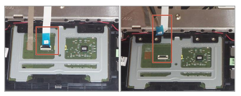
• Use a pair of tweezers to disconnect the <u>ZIF connector</u> securing the trackpad ribbon cable. Gently lift the black tab up, and the cable should come free.
