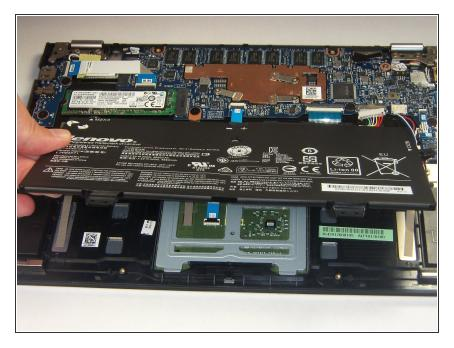
Carefully remove the battery from the device.
