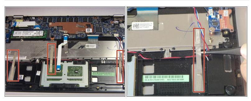
• Use a pair of tweezers to peel up one side of each of the 3 pieces of tape that cover the speaker wires.
