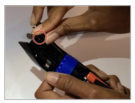
Locate the zoom lock precision notch in the back panel of the Beardtrimmer
