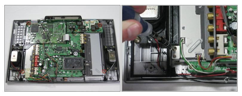
• Remove the four 5mm phillips screws attaching the LCD and circuit board to the front case.
