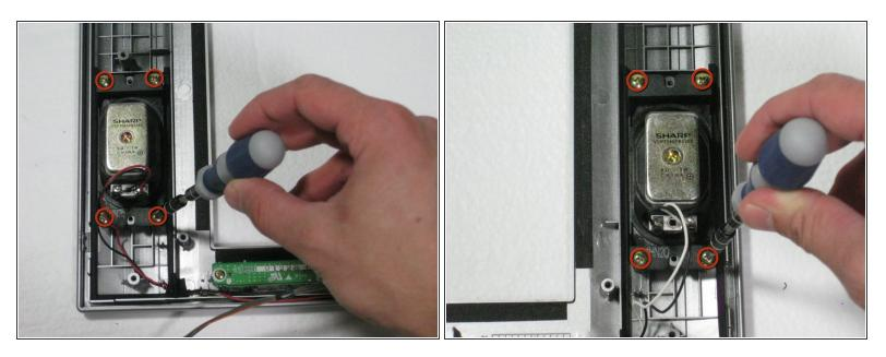
• Remove the eight 10mm screws connecting the two speakers to the front case.
