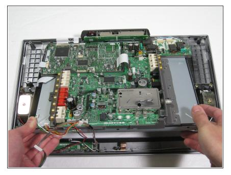
Lift the circuit board/LCD block from the case by lifting the near side of the circuit board and sliding it under the button frame.
