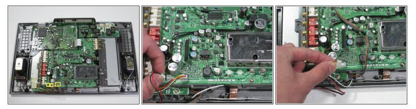
Remove the two speaker cables and the connector from the circuit board by pinching the plastic connectors and firmly pulling up.
