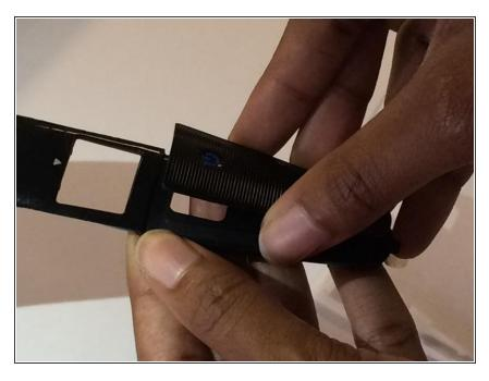
Remove the power switch from the front panel once the white plastic frame is removed.
