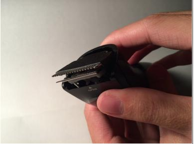
Place your thumb underneath the blade and push upward to remove it.
