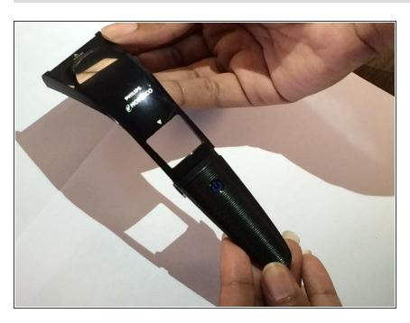
Remove the front panel completely from the rest of the beard trimmer.
