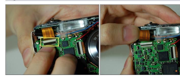
• On the front of the camera, near the flash flip, there is a connector holding a ribbon. Remove the ribbon from the connector.
