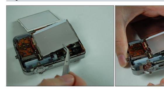
• Pry the LCD casing from the tape that is underneath it and then flip it to the opposite side to expose the contents under it.
