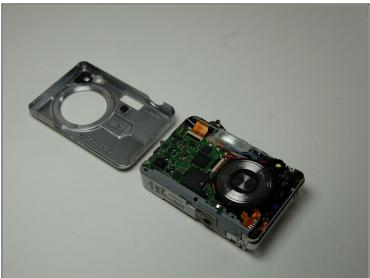
Remove the front casing from the body of the camera.
