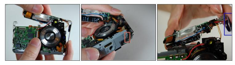
• Carefully remove the L shaped frame from the camera by popping the frame off the bumps and tabs located at the bottom of the camera.
