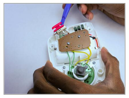
Use the plastic opening tool to remove the power button from the device.
