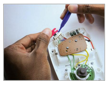
• Remove the power button from the connector and replace it.
