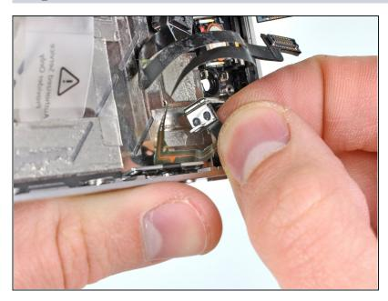
• Gently pull the silent switch bracket away from the outer case and peel its small ribbon cable off the inside of the iPhone.
