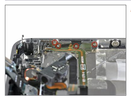
Remove the four 1.6 mm Phillips screws securing the volume button and silent switch brackets to the outer case.
