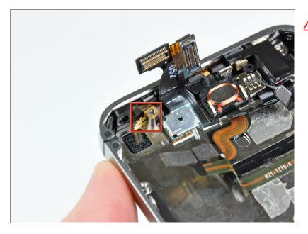
A Be sure not to lose the small grounding finger for the rear facing camera near the power button.
