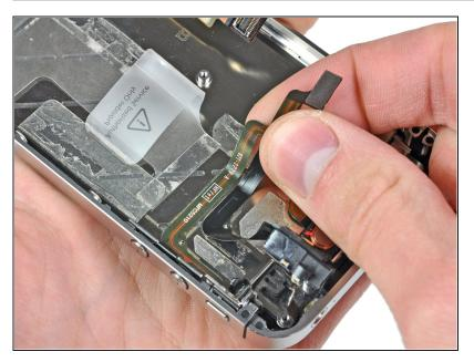
• Carefully peel the headphone jack/volume button cables off the adhesive securing them to the rear case.
