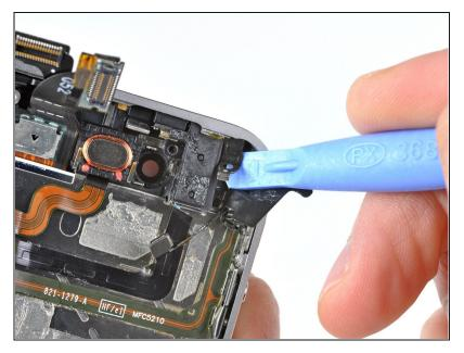
• Use the edge of a plastic opening tool to gently move the top antenna contact away from the headphone jack.
