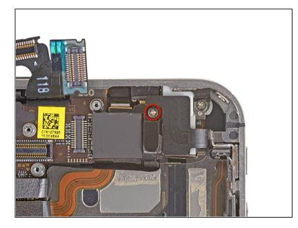
Remove the 1.5 mm Phillips #000 screw near the headphone jack.
