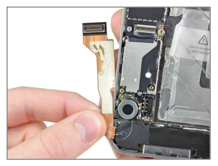
• Peel the dock connector cable off the adhesive securing it to the logic board and the side of the speaker enclosure.
