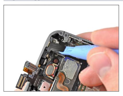
• Use the edge of a plastic opening tool to peel the upper antenna off the headphone jack.
