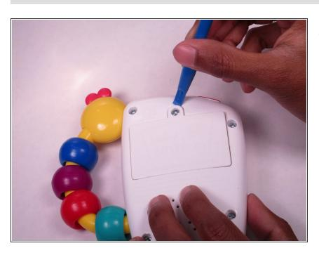
Remove the battery plate with a plastic opening tool and set it aside.
