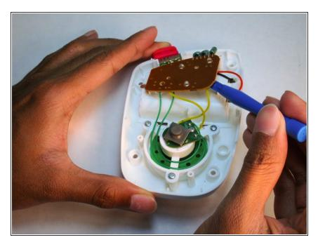
Use the plastic opening tool and carefully set the LED panel to the side, exposing the wires underneath.
