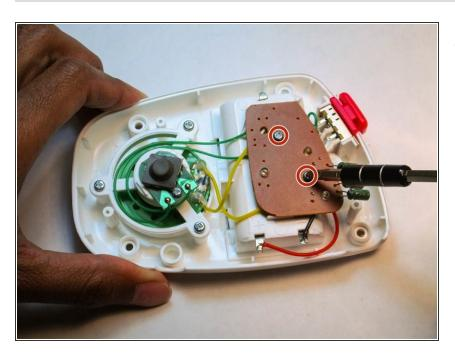
Remove the highlighted screws using a Phillips #1 Screwdriver.
