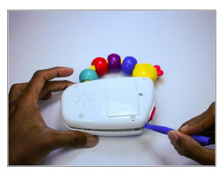
Separate the device in two parts by using the plastic opening tool.
