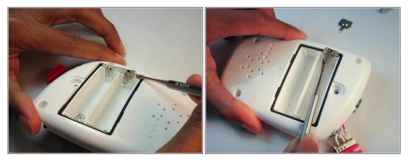
Flip the device on its face and remove the battery terminals with a metal spudger.
