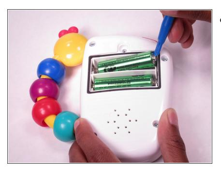
Remove each battery with a plastic opening tool and set them aside.
