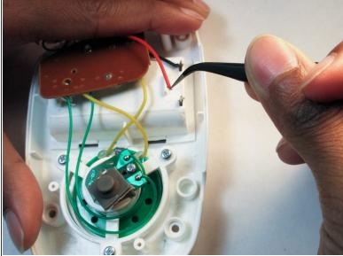
• Sever the red wire from the metal connector with the precision tweezers.
