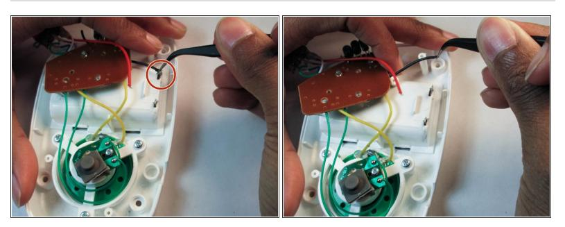
Sever the black wire from the metal connector with the precision tweezers.
