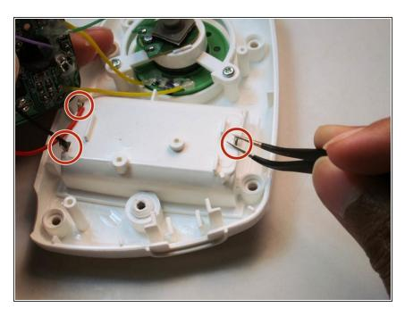
With the precision tweezers, straighten the metal connectors to remove the terminals from the other side.
