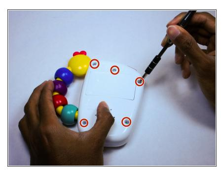
Begin by removing all highlighted screws with a using a Phillips #1 Screwdriver.
