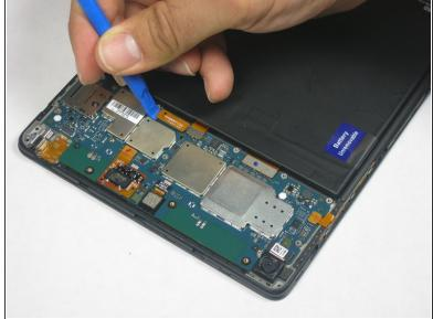
• Disconnect the six ribbon cables attached to the motherboard using a plastic opening tool.
