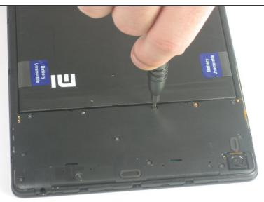
Remove the twelve 3 mm Phillips #00 screws on the upper cover of the device.
