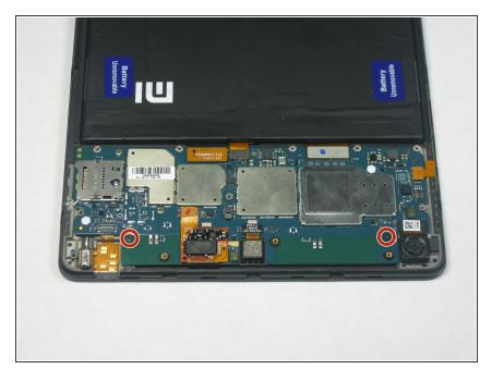
Remove the two 3.0 mm Phillips #00 screws securing the motherboard to the device.
