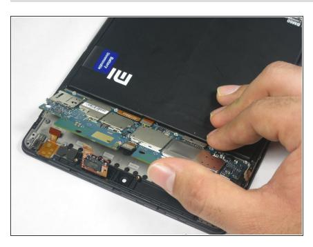
Carefully remove the motherboard from the device.
