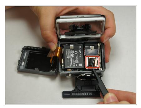
Using tweezers, peel off the copper tape on the right side of the battery.
