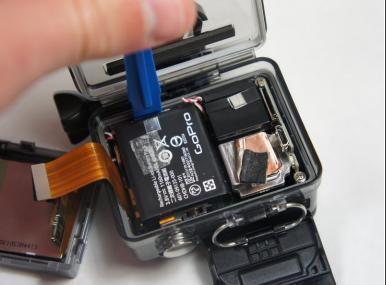
Place the plastic opening tool at one of the edges of the battery then pry until the battery is removed from the GoPro.
