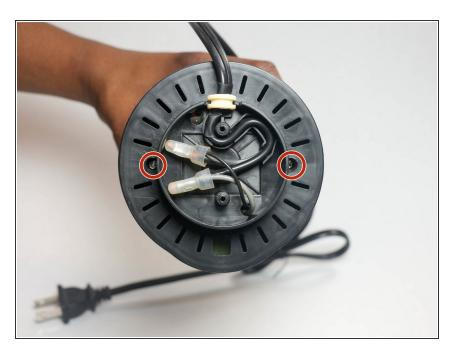
Using a Phillips #2 screwdriver, remove the two 5 mm Phillips screws from the motor platform.
