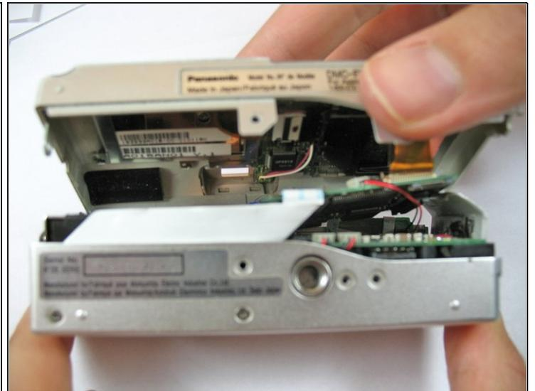
⚠ Be careful not to damage the ribbon cable when opening. Ensure it is still attached.
