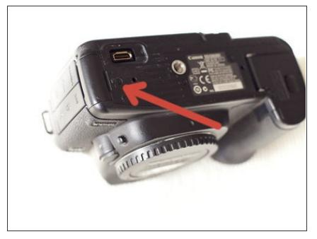
undo screw near the letter 'o' from 'open' that's indicated on the bottom left of the camera
