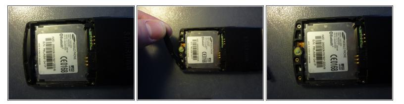
after removing the battery, remove the five small Phillips-head screws with a #0 Phillips screwdriver.
