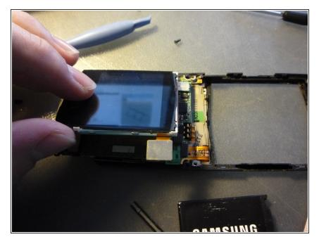
the last step is to take of old lcd from main board. mine was easy to go, but probably it could be stuck with the glue and i recommend to use a blade carefully.
