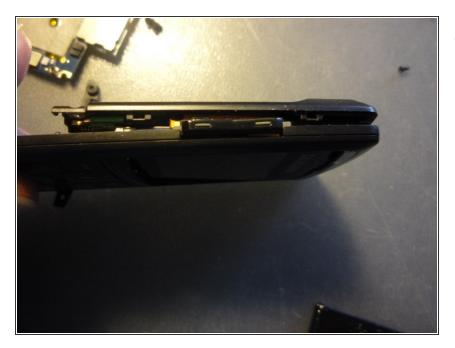
be carefull. the phone is thin and you should push on two hooks two open cover case.
