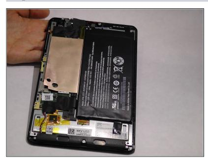
• Turn the tablet over so the battery is facing up.
