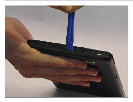
Begin prying the front from the back on any side of the tablet. Gently work your way around the tablet with the prying tool.
