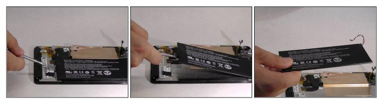
• Using a <u>plastic card</u> or opening pick, separate the battery from the rest of the device.
