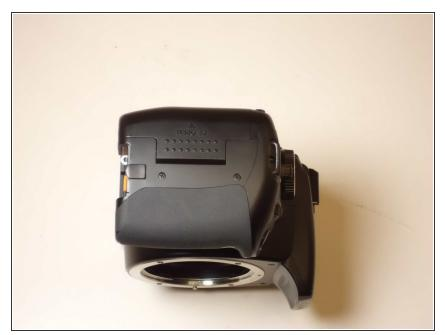
Place the camera on its side with the soft touch grip facing up and the top of the camera facing right.
