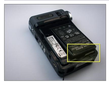
Take the battery out by pulling up on the bottom of the battery. You should be pulling from the side of the camera where the wrist strap is attached.
