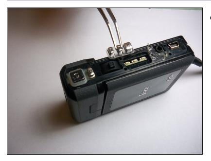
Remove the three combined buttons so they are not misplaced.
