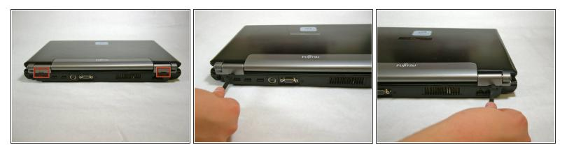
• Use a spudger to lift the back of the hinge cover on the left and right sides of the computer.
