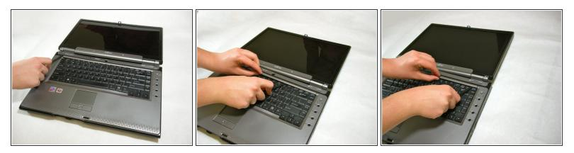
• Use a spudger to partially lift the hinge cover.
