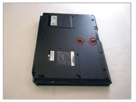
Locate the two clips on the bottom of the computer that support the battery.
