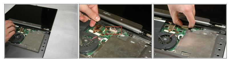
• Use a spudger to detach and remove cables from the motherboard.
