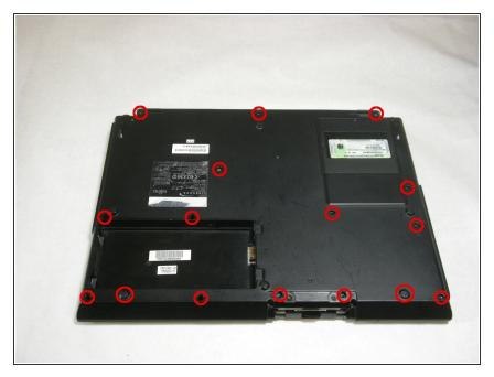
• Remove screws from bottom of laptop as shown in the picture.
