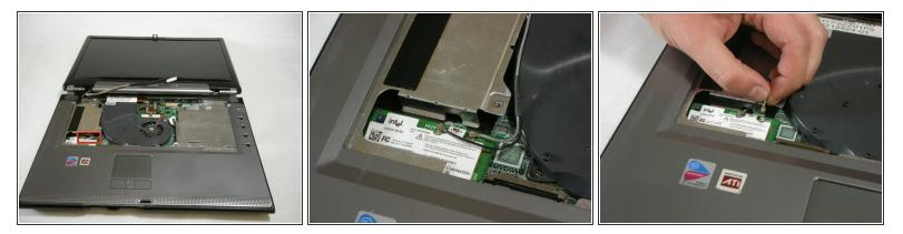
• Unplug highlighted cables from the wireless module.
