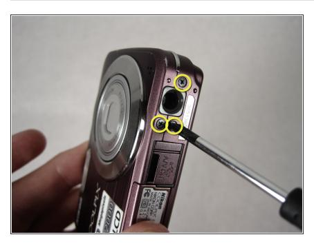
Unscrew the three 4.05mm screws on the bottom of the camera below the lens.
