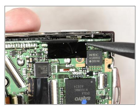
Place the spudger underneath the small black tape as shown. Gently lift the spudger up to remove the tape.
