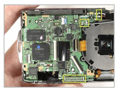
Desolder the marked areas. For desoldering instructions go -here-
