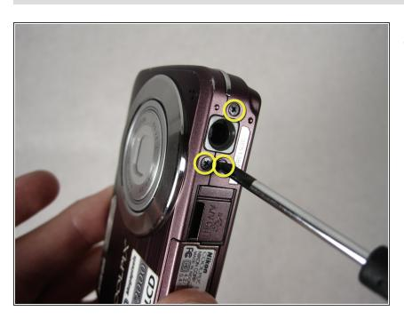
Unscrew the three 4.05mm screws on the bottom of the camera below the lens.
