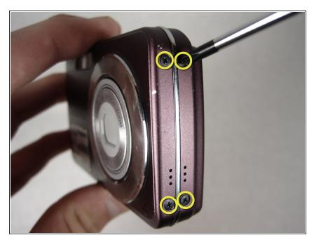
After removing the battery, unscrew the four 3.10mm screws on the side opposite the buttons.
