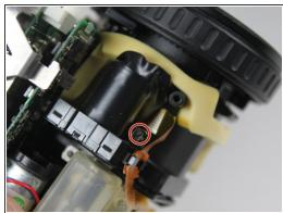
Remove all three screws around the lens assembly.
