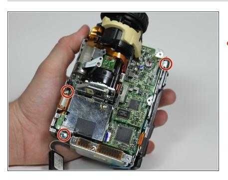
Remove the three screws from the circuit board.
