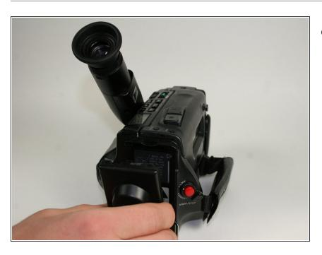
Pull the battery pack out of the video camera.
