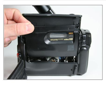
Pull off the plastic tape cover by lifting it up and out of the camera base.
