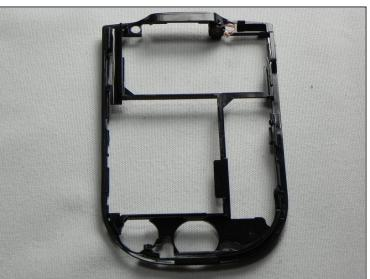
• Finally the mother board can be removed from the center black frame.
