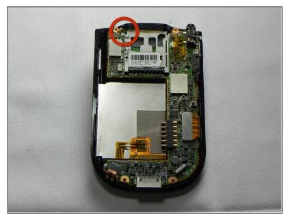
Now that the back cover is removed, use the #00 Philips x .17 screwdriver to remove the small screw to the left of the SD card slot.
