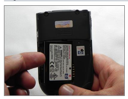
Now, lift the battery up and away from the device to remove it.
