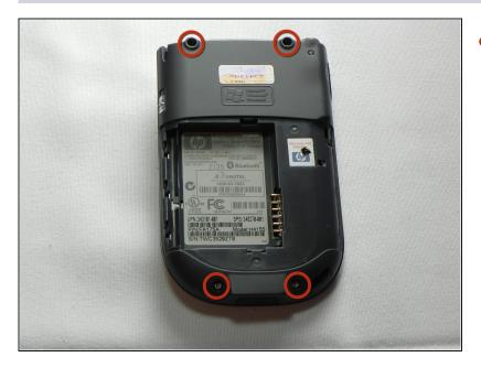
• Remove the four silver screws using the T5 Torx Screwdriver (T5 x .25 in).
