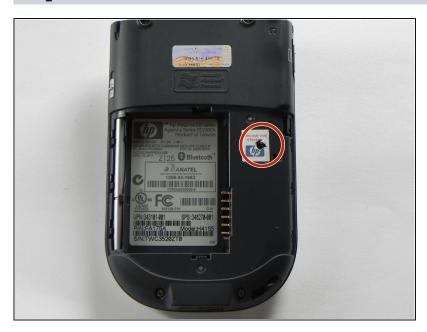
Remove the single black screw that is located beneath the HP sticker with the T5 Torx Screwdriver.
