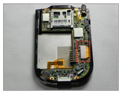
Now that the front cover is removed we will need to disconnect the LCD screen from the mother board. Pull the LCD connection out of the slot to properly disconnect.
