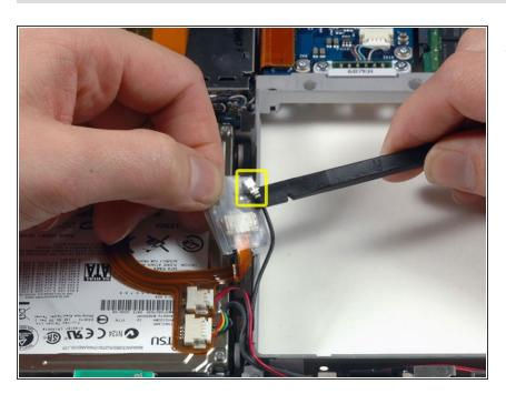
Lift the Bluetooth board out of its slot next to the hard drive and use a spudger to disconnect the Bluetooth antenna cable.
