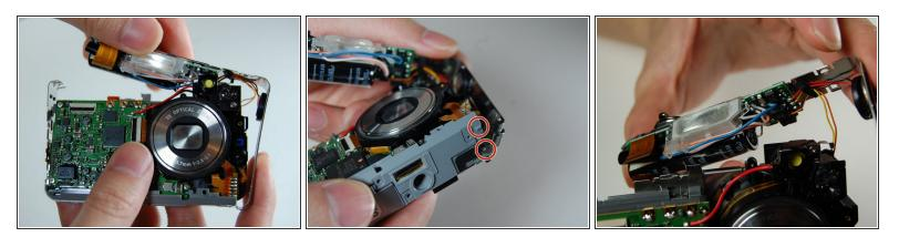
• With the lens facing towards you, pull the L-shaped frame away from the camera.
