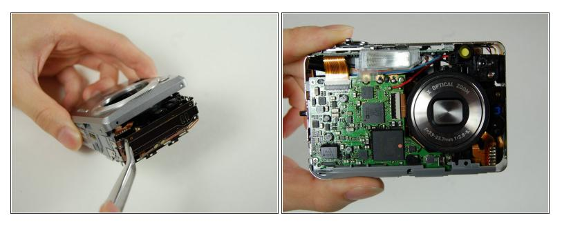
• Use your tweezers to hold the camera secure, while you pull the front cover off of the camera.
