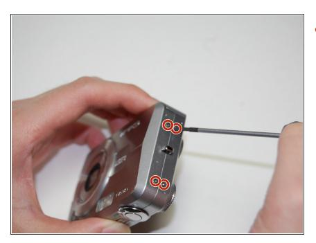
Use a Phillips #00 screwdriver, unscrew all four screws on the left side of the camera.
