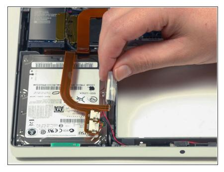
Slide the Bluetooth board out of its slot next to the hard drive. The Bluetooth board is still connected to the orange hard drive cable, so don't try to remove it entirely from the computer.
