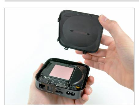
Carefully remove the bottom cover from the unit
