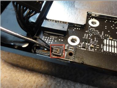
Using a screwdriver (flathead) or a spudger, pull the power cable out of the logic board
