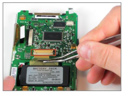
Using the same technique as with the other ribbons, locate and disconnect the ribbon cable above the battery pack.
