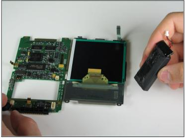
• Wedge the spudger under the battery to pry it apart from the adhesive.
