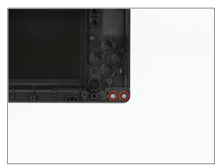
Remove the two 8.3 mm Phillips screws securing the upper case to the display assembly.
