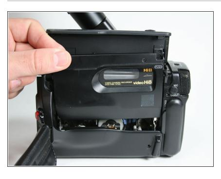
Pull off the plastic tape cover by lifting it up and out of the camera base.
