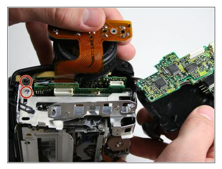
Remove two remaining 3.6 mm case screws from the front of the camera.
