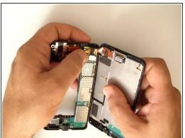
Put the earpiece on the new display assembly and start with reassembling.
