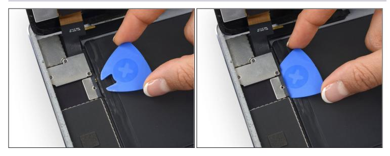
⑦ To reduce the risk of a short, you can use a battery isolation pick to disconnect the battery.
