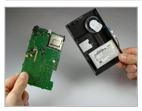
Lift the motherboard out of the outer case.
