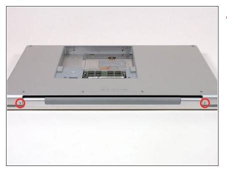
Rotate the computer 90 degrees and remove the two 3.2 mm Phillips screws from the rear of the computer.
