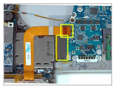
• Disconnect the hard drive and ExpressCard connectors from the left side of the logic board.
