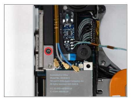
Remove the single black T6 Torx screw located just above the Airport Extreme card.
