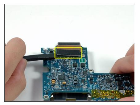
• Turn the left I/O board over and disconnect the short left I/O board cable.
