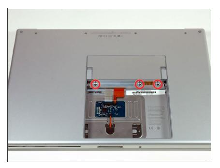
• Remove the three identical Phillips screws from the memory door.
