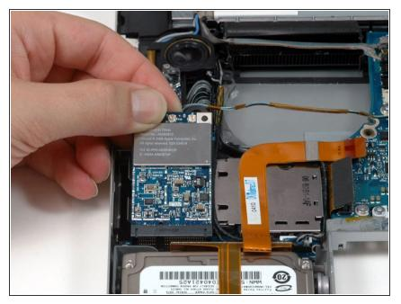
• Lift the Airport Extreme card up and slide it out of its connector.
