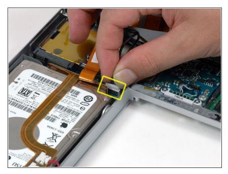
• Disconnect the speaker cable from the corner of the left I/O board.
