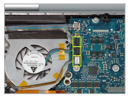
Disconnect the inverter, left fan, and left ambient light sensor cables by placing a spudger beneath each cable and lifting up.
