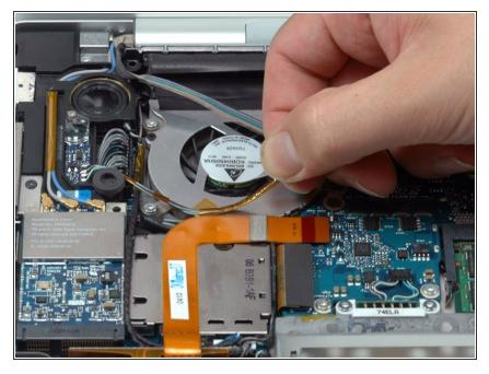
• Peel up the left ambient light sensor cable from above the left fan, removing tape as necessary.
