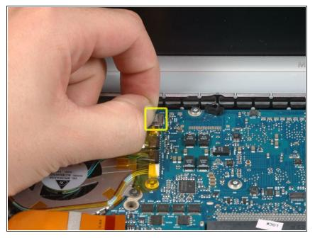
• Disconnect the iSight cable from the logic board by sliding the cable to the left and out of its connector.
