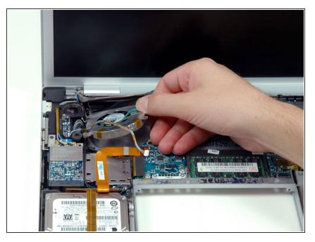
• Lift the left fan up and carefully peel up the tape securing the fan to the heat sink as you go.
