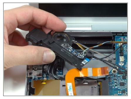
• Lift the left speaker assembly out of its housing and place it in the area previously occupied by the left fan.
