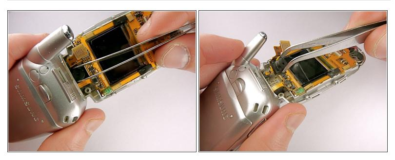
Using tweezers, remove the camera from the cellphone casing.
