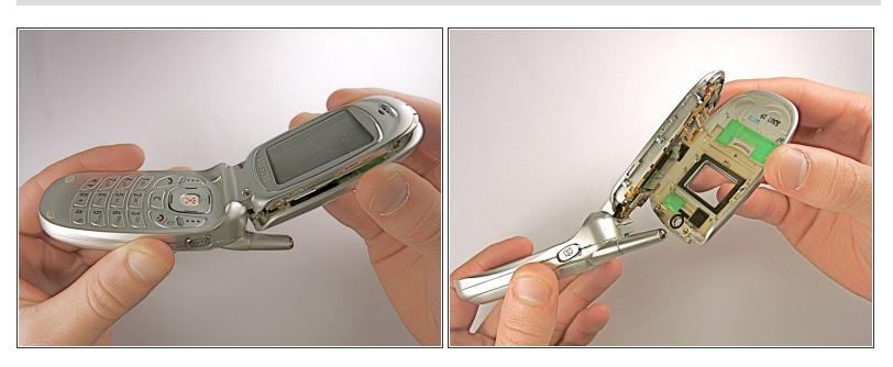
Make sure that the top panel is completely separated from the LCD display around the entire perimeter.
