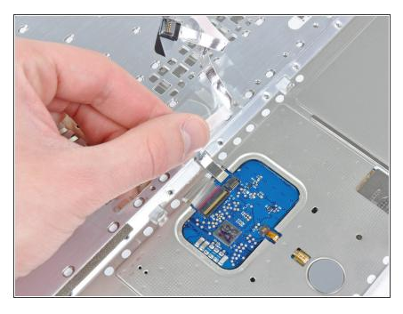
Pull the upper case cable out of its socket and remove it from the upper case. To reassemble your device, follow these instructions in reverse order.
