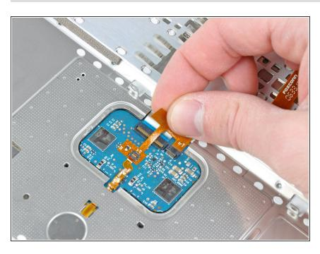
Gently peel up the section of the upper case cable stuck to the keyboard ribbon cable, being careful not to disturb the keyboard ribbon cable in the process.
