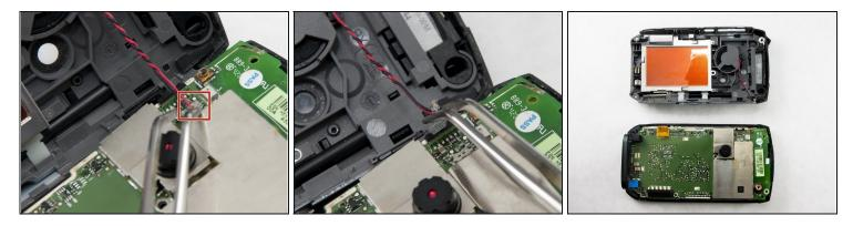
• Using <u>tweezers</u>, squeeze the plastic head of the black and red wound wire cable. This will detach the cable from the circuit board and fully separate the two halves.
