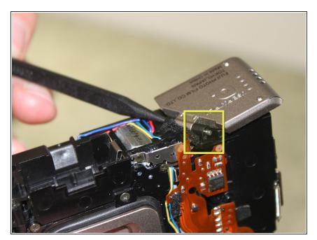
Push the pin from one side with the spudger until it comes out on the opposite side.
