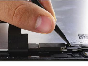
• Use the flat end of a spudger to flip up the retaining flap on the Home Button cable socket.
