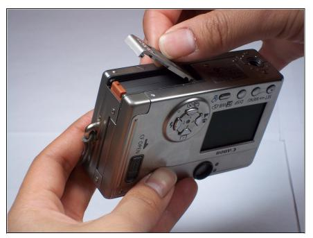
Hold the end of the battery cover that extends beyond the camera and lift it up.
