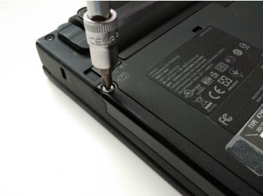
Unscrew the HDD slot cover.
