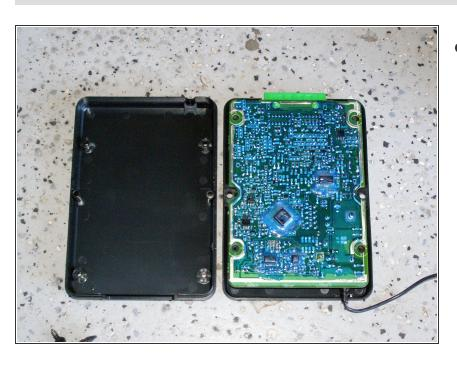
Remove the 4 screws (may be under the foam strips). This is the bottom of the circuit board.
