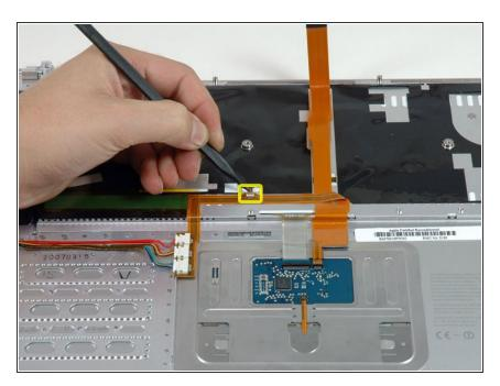
Use the tip of a spudger to flip up the brown plastic flap locking down the keyboard backlight ribbon cable.
