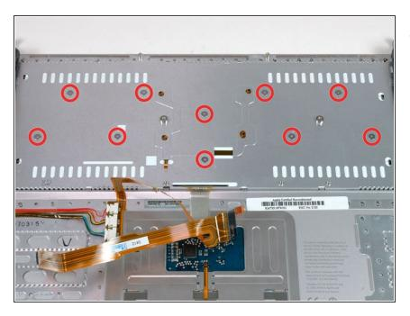
Remove the ten identical Phillips screws attaching the keyboard to the casing.
