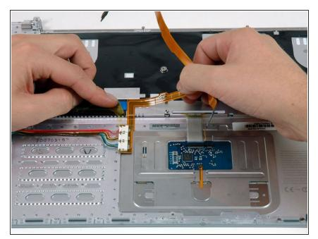
Carefully peel up the orange ribbon cable which carries the power and sleep signals, removing tape as necessary.
