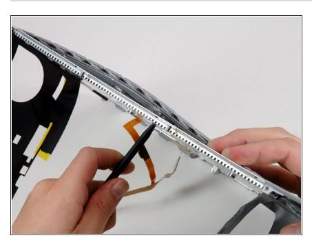
Place the upper casing on its edge and use a spudger to push the keyboard away from the casing, poking the spudger through the central keyboard screw hole. Grasp the keyboard as it separates from the casing.
