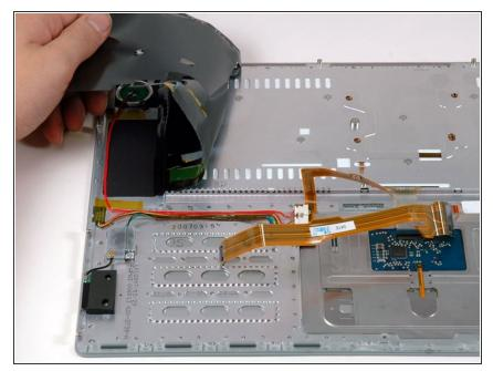
Peel back the black protective sheath on the left side of the upper case. It is not necessary to fully remove this shield. Simply peel it back enough to access the screws beneath.
