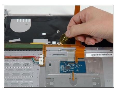
Peel up the orange tape covering the keyboard backlight connector.
