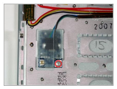
Remove the single Phillips screw securing the Bluetooth board to the lower case.
