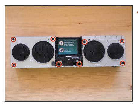
Remove the eight Phillips screws securing the front cover to the back cover.
