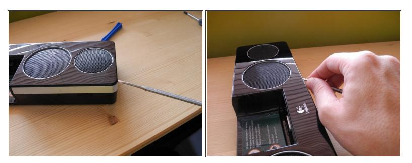
Now work your way along all sides, cuting through the glue with the spudger. The glue is all over so make make sure to go deep enough under the cover with the spudger.
