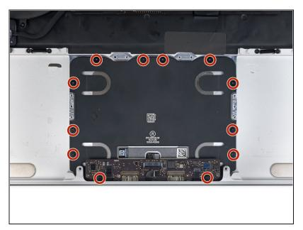
Remove the twelve 2.4 mm T5 screws securing the trackpad to the upper case.
