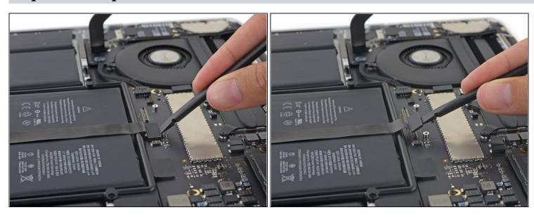
Use the flat end of a spudger to pop the trackpad connector straight up off its socket on the logic board.
