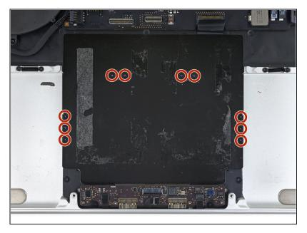
Remove the ten 2.8 mm T3 screws securing the trackpad cover plate to the upper case.
