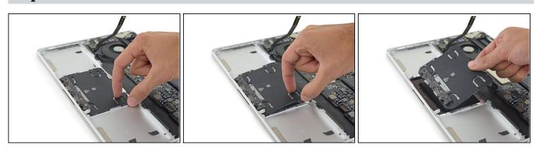
Lift up and remove the trackpad from the upper case.
