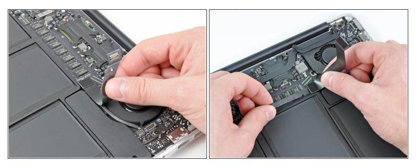
The following connector has an especially deep socket. Use care when disconnecting it.
